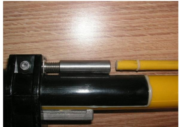
Rod section marked "A" above separated from the coupling marked "B" above. The product specification sheet from Salisbury indicates that a pin should have been installed in the coupling (B) to hold the rod in place.
